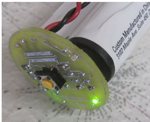
Figure 16 - Torpedo control circuit
