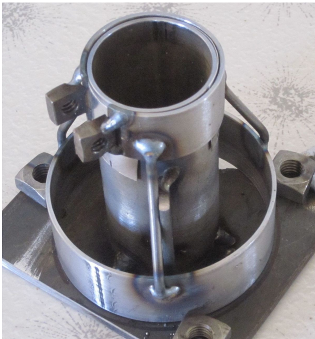
Figure 3 - Thruster welding jig
